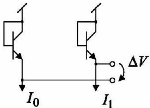
$$\frac{\Delta V}{V_T} = \frac{V_0 - V_1}{V_T} = 2 \tanh^{-1} \left( \frac{\Delta I}{I} \right) = L(X)$$
