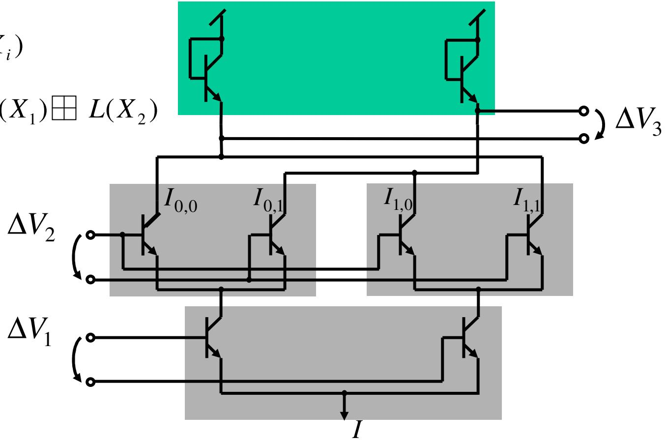
$$\frac{\Delta V_3}{V_T} = 2 \cdot \tanh^{-1} \left[ \tanh \left( \frac{\Delta V_1}{2V_T} \right) \cdot \tanh \left( \frac{\Delta V_2}{2V_T} \right) \right]$$
